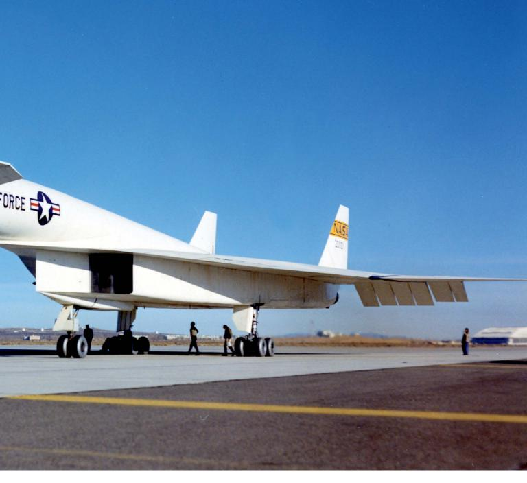
of hypersonic flight. It was manufactured using a brazing process, a technique that became widely used throughout the aerospace industry, rather than being welded.
