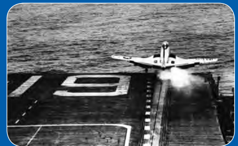
PHOTO: This F2H-3 Banshee was the first jet fighter to launch off the deck of an aircraft carrier, the USS Hancock , using a steam catapult. BOEING ARCHIVES
