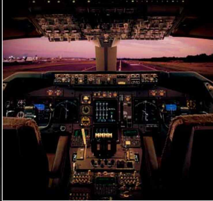
PHOTOS: (Above) The advanced flight deck of the 747-8 contains new technology, but it is similar enough to the 747-400 that pilots rated for that airplane can be rated for the 747-8 with minimal training. BOEING
