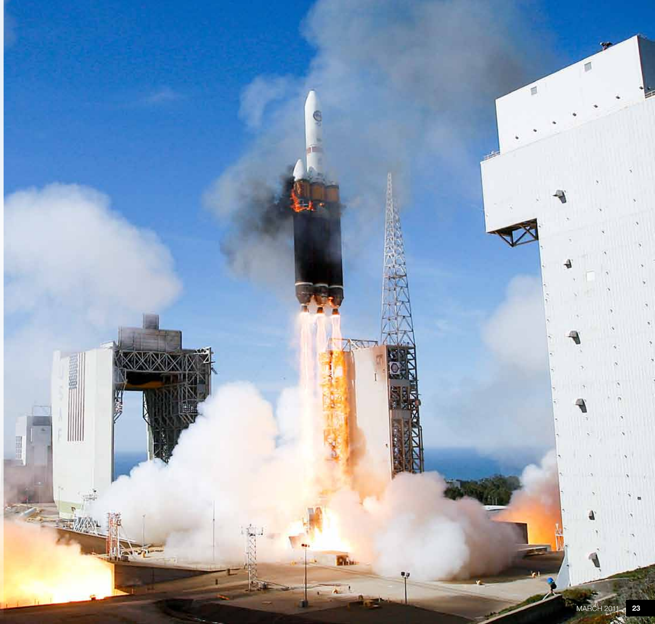
PHOTOS: (Right) The Delta IV Heavy soars skyward from its launch pad near the Pacific Ocean. The flames near the top of the booster on the left are from liquid hydrogen vapors being burned off and are not unusual. ASSOCIATED PRESS (Inset) The massive Delta IV before launch. UNITED LAUNCH ALLIANCE
