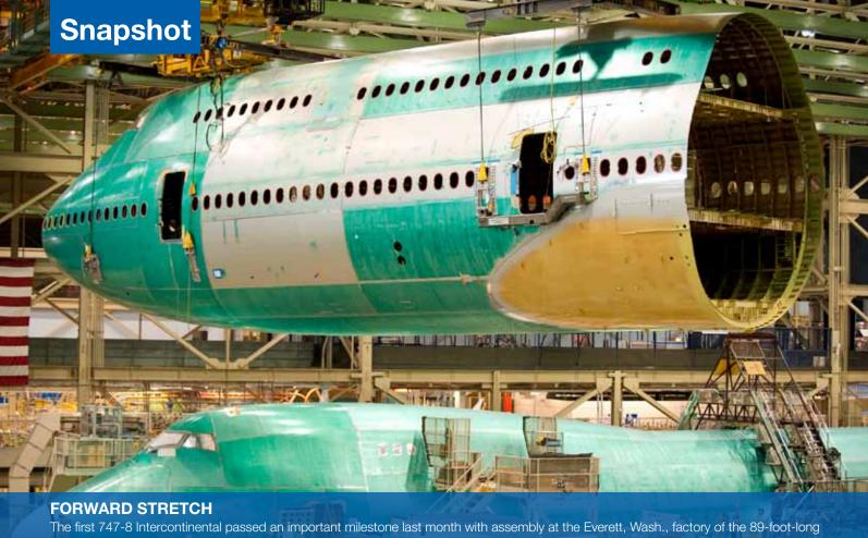
The first 747-8 Intercontinental passed an important milestone last month with assembly at the Everett, Wash., factory of the 89-foot-long (27.2-meter) forward fuselage, including the upper-deck passenger cabin. The 747-8 is 18 feet 4 inches (5.6 meters) longer than the 747-400, with much of that added length in the forward fuselage, seen here with a 747-8 Freighter in the background. TIM STAKE/BOEING
