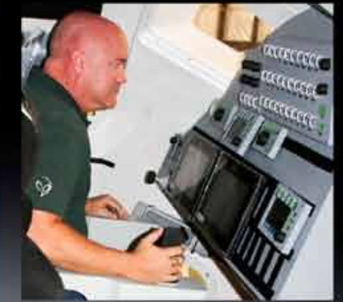
PHOTOS: (Below) Leslie Robertson, Boeing Software Engineering, and John Wissinger, Boeing Space Operations and Ground Systems, run a simulation in the Avionics Systems Integration Facility in Houston to support rapid prototyping of avionics systems and full-scale avionics systems development for the Boeing CST-100 spacecraft. ELIZABETH MORRELL/BOEING (Insets, from left) Bill Overton, Boeing technology support subcontractor, Mike Fraietta, Boeing Space Operations and Ground Systems, and John Gasvoda, Boeing Software Engineering, participate in a simulation run in the Avionics Systems Integration Facility. ELIZABETH MORRELL/BOEING A test of the CST-100 airbags, which are used to upright the vehicle in case it inverts after an emergency water landing. BIGELOW AEROSPACE Bigelow Aerospace program manager Tom Londrigan performs tests in the full-scale CST-100 mock-up. BIGELOW AEROSPACE
