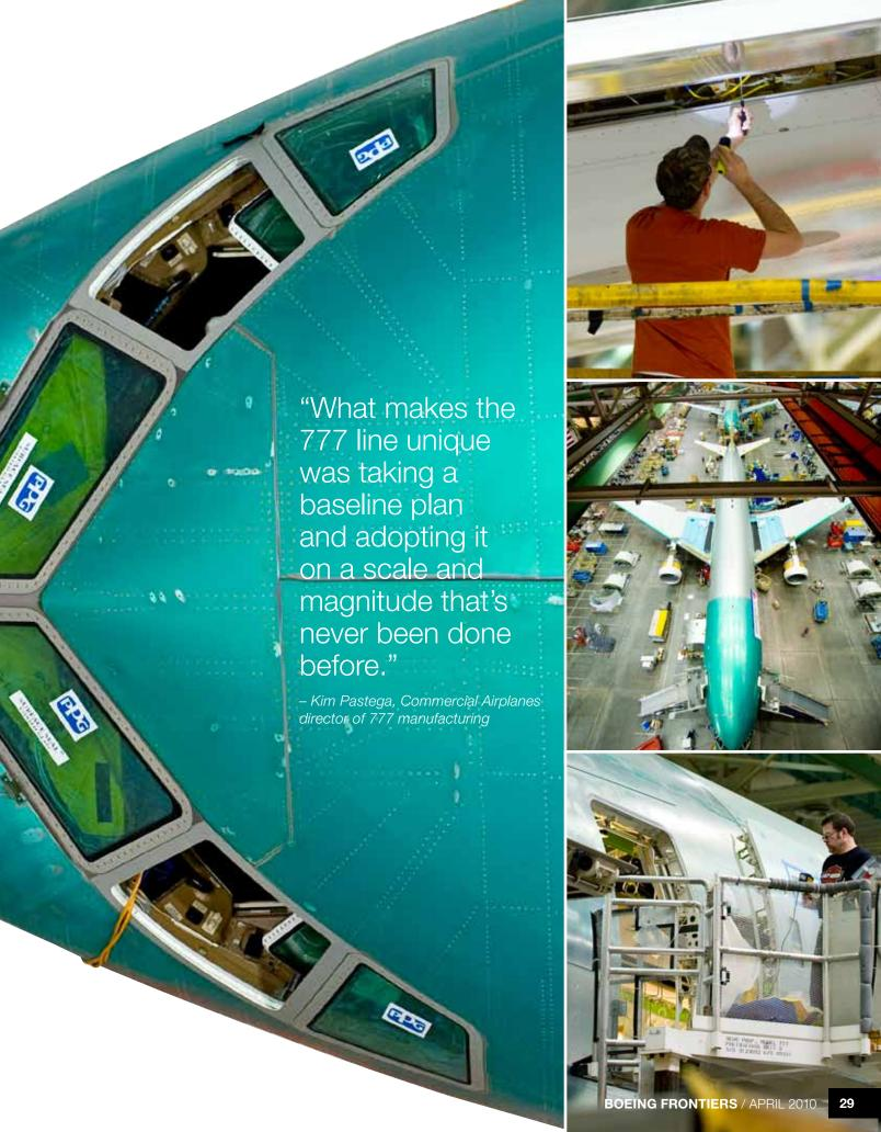
assembled. The 777 line is believed to be the most extensive moving production line used to build a commercial airplane. A new, empty 777 weighs 366,940 pounds (166,441 kilograms) and includes about 3 million parts.
