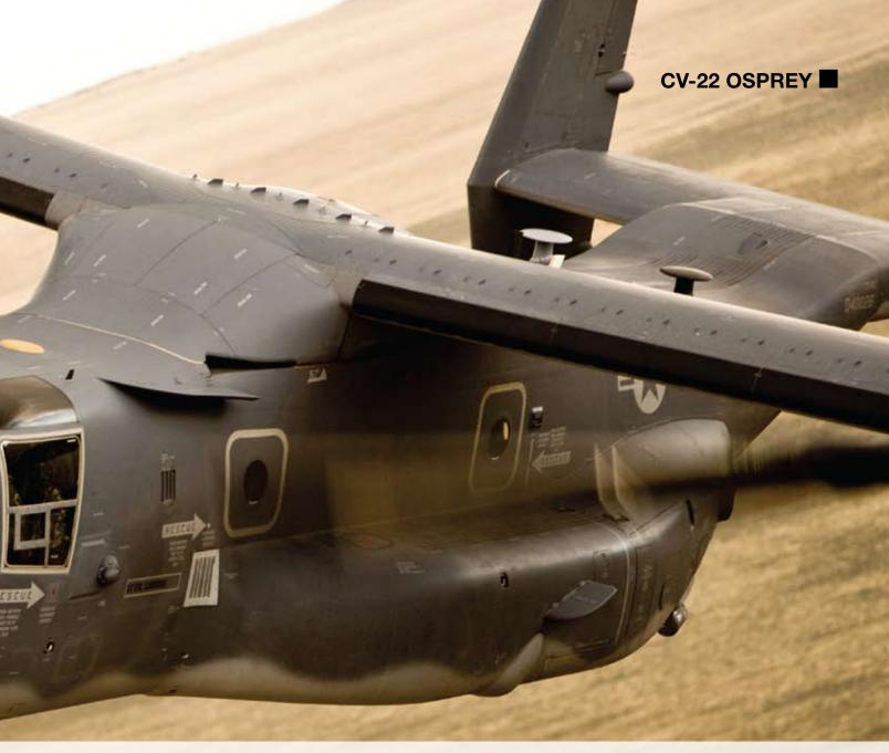
according to Boeing officials. Like a helicopter it can land in areas that aren't prepared for fixed-wing aircraft, putting troops and supplies exactly where they are needed with no need for a runway. It also can deliver 24 combat troops and sizable amounts of supplies. This includes up to 20,000 pounds (9,070 kilograms) of internal load and the ability to sling-load, or carry underneath the aircraft, as much as 15,000 pounds (6,800 kilograms).
