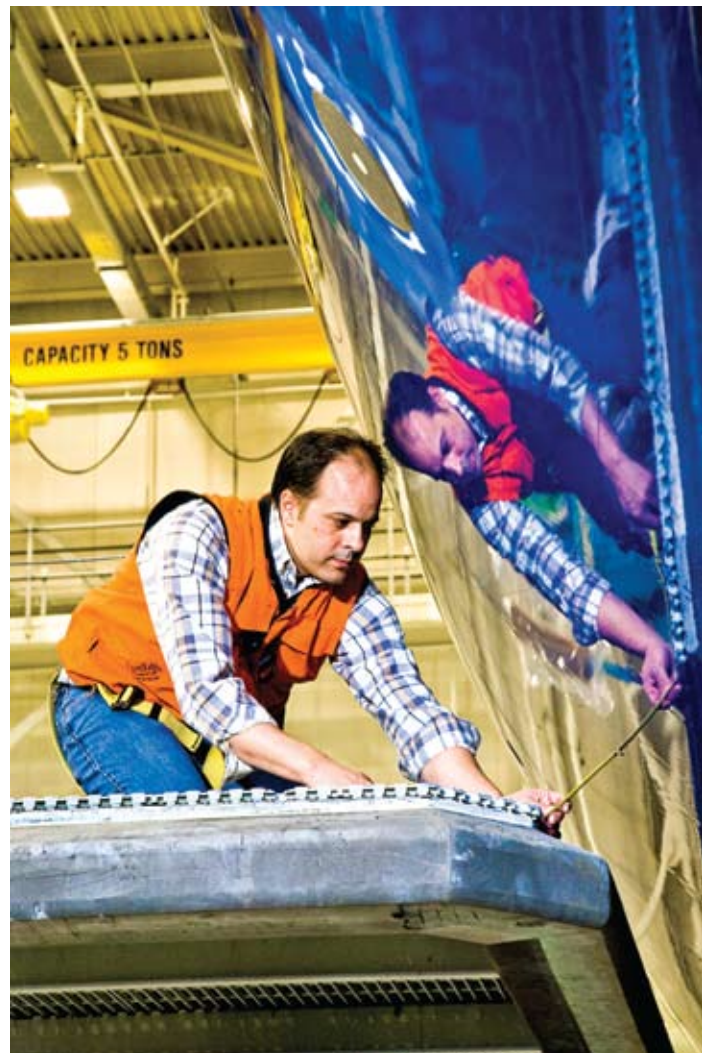
PHOTO: Everett Site Services Plant Engineering automation designer Neil Kuntz works on one of the 45-03 paint hangar's crane stackers during the collision avoidance calibration process. The stackers are overhead hoisting platforms that painters operate and ride to allow access to the entire surface of the airplane.
