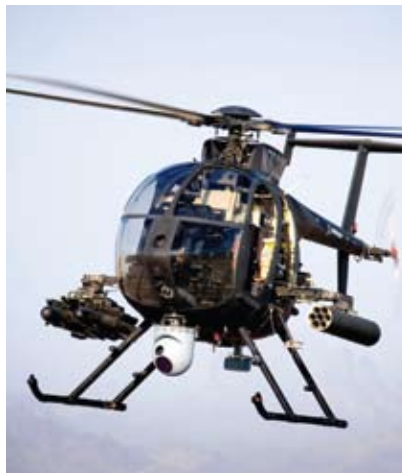
PHOTO: The AH-6U Unmanned Little Bird can be configured as an unmanned or manned platform for operations in complex or urban terrain.
