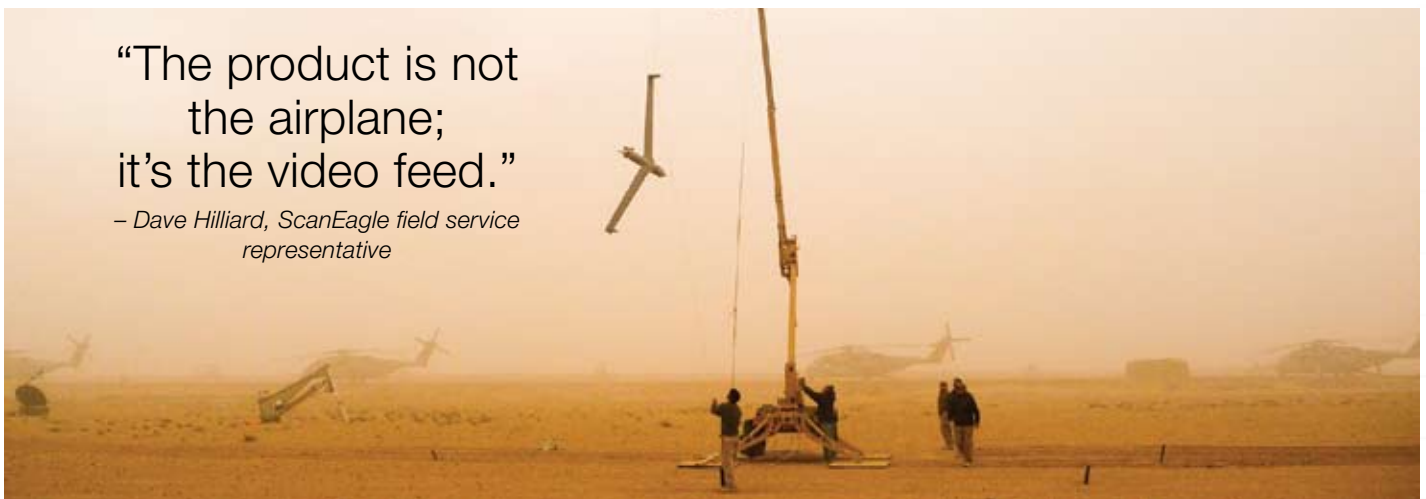
PHOTO: Dave Hilliard (foreground), a Boeing field service representative, retrieves a ScanEagle after its capture on the Skyhook system as another haboob (sandstorm) closes in on Al Asad Air Base, Iraq. ERIC MALMGREN/INSITU
