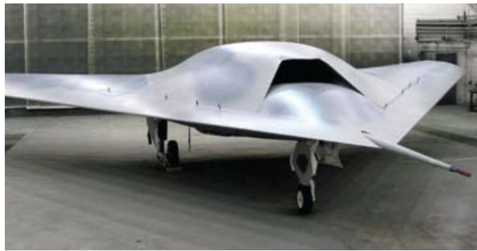
PHOTO: Based on the fighter-size X-45C airframe, Phantom Ray is being used to rapidly prototype an expanded flight envelope and unmanned combat missions capability. BOEING
