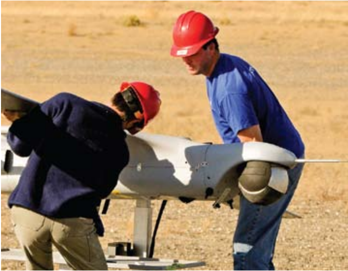
PHOTO: Insitu engineers Andy Mack (left) and Wayne Larson prepare to flight-test a prototype of Integrator, a larger, twin-boom derivative of ScanEagle. PETER KUNZ/INSITU
