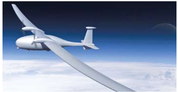
GRAPHIC: The High Altitude Long Endurance system, designed to take on border surveillance, port security and telecom missions at 65,000 feet (19,800 meters) and higher, will stay aloft for seven-plus days on liquid hydrogen fuel-cell propulsion. BOEING
