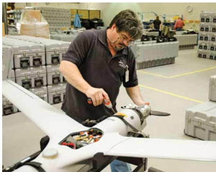
PHOTO: Jim McClanahan, Insitu production shop team lead, secures the engine fairing on a ScanEagle, one of many Boeing programs that rely on radio-frequency spectrum. DOUG CANTWELL/BOEING
