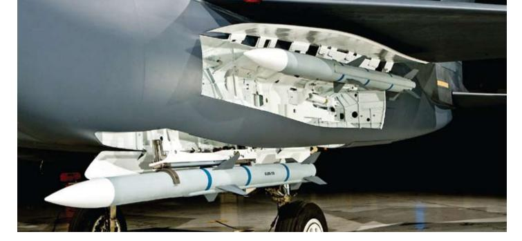
New components include conformal fuel tanks with internal weapons bays, called conformal weapons bays, that have the same aerodynamic shape and aircraft interfaces as the standard conformal fuel tanks of the F-15E. Conformal fuel tanks are additional fuel tanks fitted closely to the profile of an aircraft, which extend either the range of an aircraft or the time on station, with little aerodynamic penalty compared to the same fuel capacity carried in external drop tanks.
