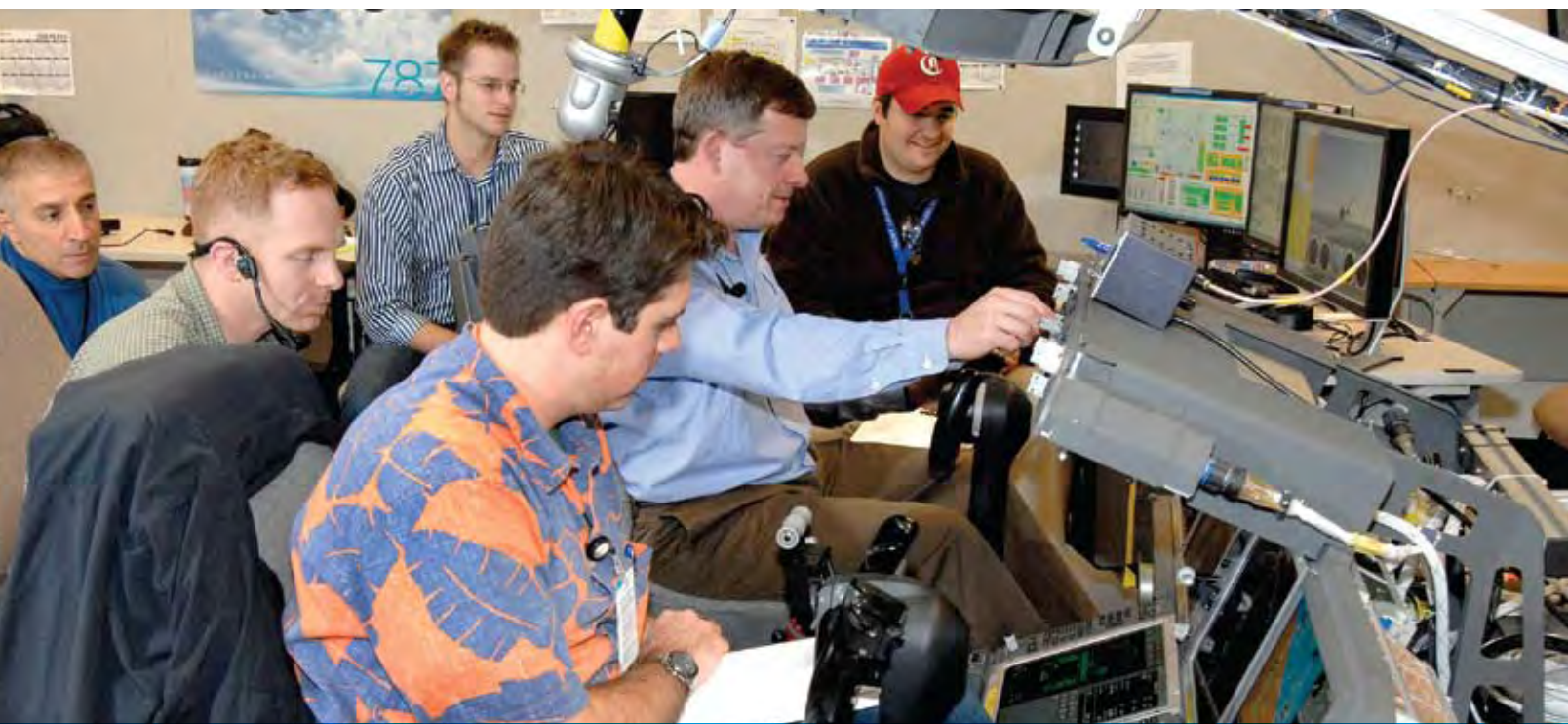
Mike Bryan (second from right), 787 project pilot, conducts a flight test in the ZA000's flight deck simulator while test engineers and analysts monitor performance. From left: Cameron Ghahreman, Tyler Finn, Matt Lassen, Christopher Caps, Bryan and Tim Cassady. When the first 787 takes flight, ZA000 will takeoff in the lab and shadow the initial flight. JIM ANDERSON/BOEING
