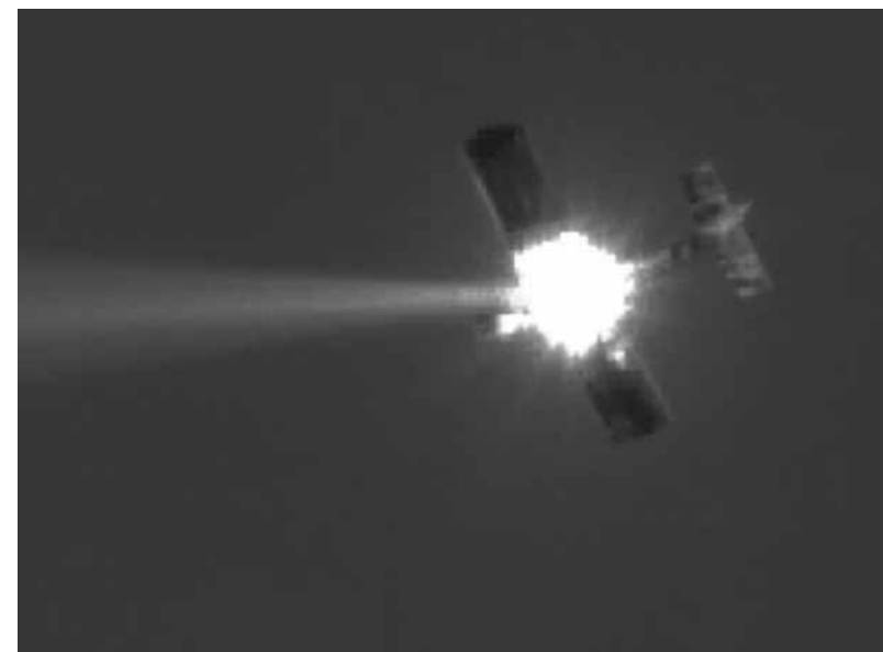
PHOTO: An unmanned aerial vehicle is hit by the high-energy laser beam fired from a Boeing-developed, trailer-mounted test bed known as the Mobile Active Targeting Resource for Integrated eXperiments, or MATRIX. U.S. AIR FORCE RESEARCH LABORATORY
