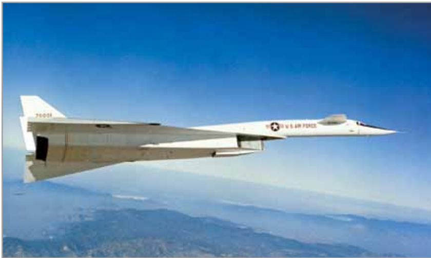
PHOTO: The XB-70 Valkyrie bomber prototype achieved speeds above Mach 3 (three times the speed of sound). BOEING ARCHIVES
