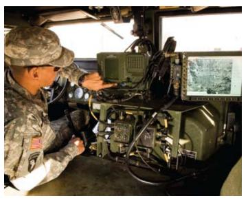
PHOTOS: (ABOVE) Inside specially equipped High-Mobility Multipurpose Wheeled Vehicles, soldiers' situational awareness is maintained through a network of sensors and robotics, increasing security for the soldiers during surveillance and reconnaissance missions. BOB FERGUSON/BOEING
