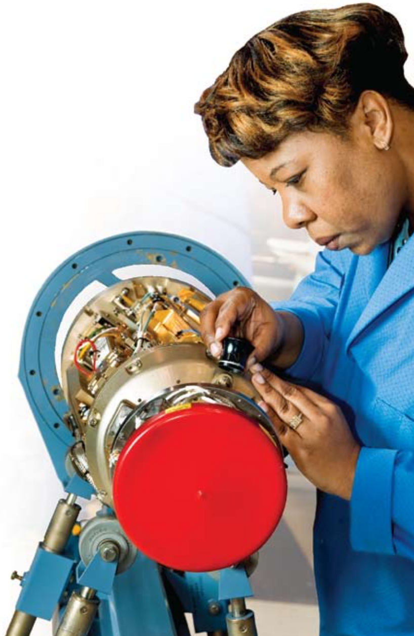
PHOTO: Integration technician Angelique Nelson completes final assembly of seekers for Patriot Advanced Capability-3 (PAC-3) Missiles.
