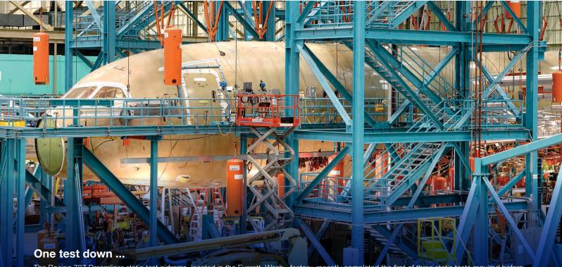
The Boeing 787 Dreamliner static test airframe, located in the Everett, Wash., factory, recently completed the first of three static tests required before first flight. During the "high-blow" test, which lasted about two hours, the airframe reached an internal pressure of 14.9 pounds per square inch (1.05 kilograms per centimeter) gauge (psig), 1.5 times the levels expected to be seen during operations. GAIL HANUSA/BOEING
