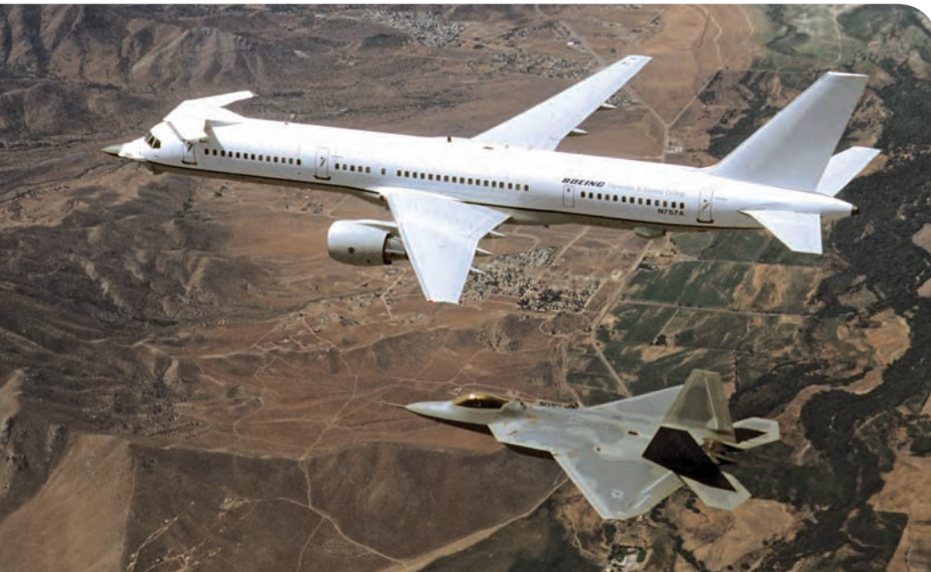
Besides flight-testing the F-22 (as he’s doing here), test pilot Chuck Killberg managed operation of the prototype 757 (shown here, above the F-22) as it was transformed into a testbed to expedite development of the Raptor’s avionics. LOCKHEED MARTIN PHOTO BY KEVIN ROBERTSON
