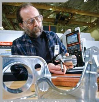
John Conant, machinist in Boeing's Fabrication manufacturing business unit located in Auburn, Wash., uses a micrometer to check parts measurements for the 777.
