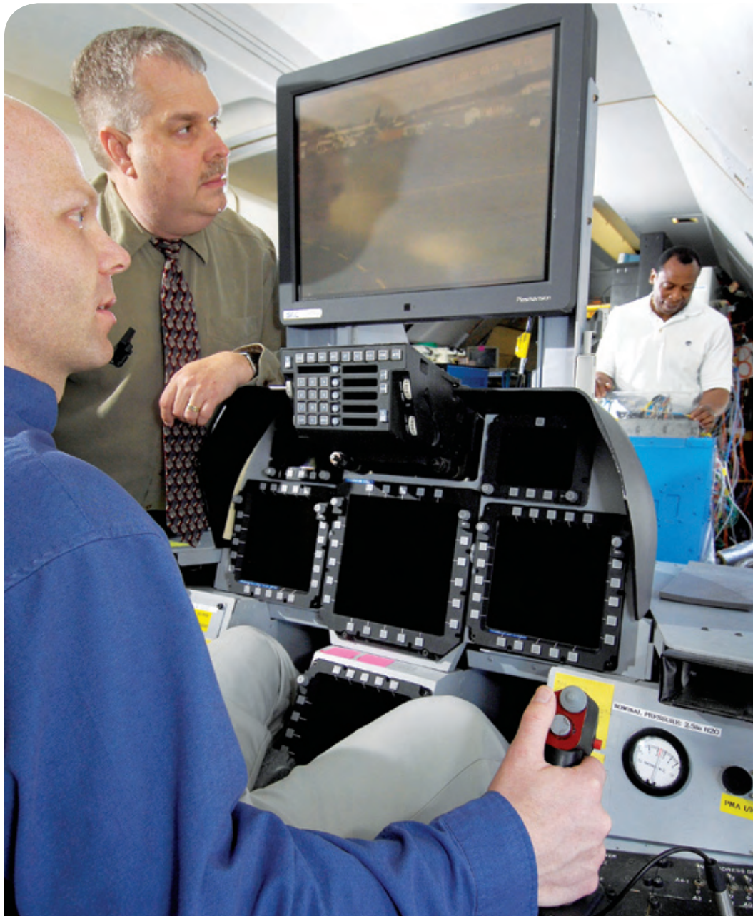
Both the 757 Flying Test Bed and the Agile Integration Lab house a full-scale F-22 cockpit. Here Brian Harden, AIL program manager (center), and Kelly Haynes, cockpit communications engineer (left), work with the FTB cockpit located in the 757’s cabin, which allows evaluation of the man-machine avionics interface under actual flight conditions.
