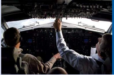
Once in flight, the pilots conduct a series of flighttest maneuvers. The crew on board-two pilots, a flight analyst and a systems operator-check systems at high and medium altitudes. They check backup and critical safety elements, including cabin pressurization and the deployment of oxygen masks, as well as avionics, navigation and communication systems, functionality of in-flight entertainment and more. They also shut down and "relight" the engines during this phase.
