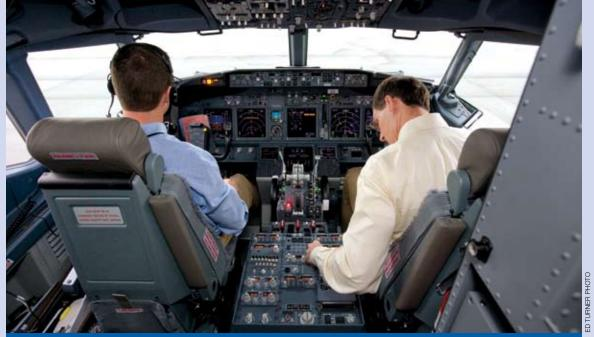
Preflight ground checks continue inside the aircraft prior to taking to the skies. Pilots Bill Mnich and John Frischkorn test airplane systems with a Ground Crew member on the tarmac at Renton Field. Tests performed during this phase include electrical system function, backup systems operation, and more.
