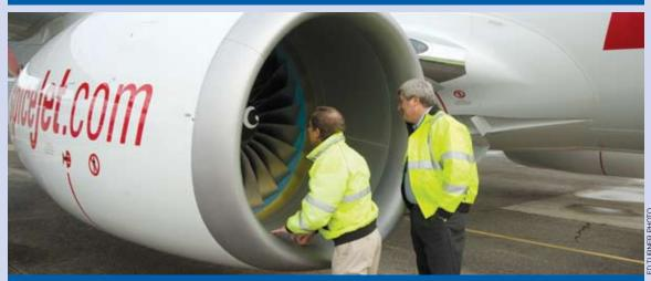
Once the test pilots have completed the necessary paperwork, they head out to the flight line to begin a series of checks outside the aircraft. Here Assistant Chief Production Test Pilot Gary Meiser (left) and Production Test Pilot Greg Guest perform a preflight inspection of a 737's engines.
