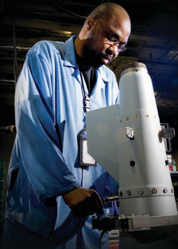
Terry Griffin torques the bolts on a Joint Direct Attack Munition Tail Actuator Subsystem (TAS) kit. The TAS helps steer the bomb to the target.
