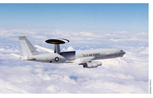
The U.S. AWACS has a flight crew of four and from 13 to 19 mission specialists aboard. The aircraft has an endurance of more than eight hours unrefueled.
