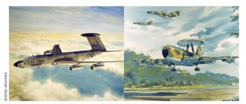
These two images show early configurations for a 707-based AWACS aircraft. The illustration on the left shows Boeing's initial configuration for the AWACS, which featured a tail-mounted rotodome mounted on a forward-swept vertical stabilizer. On the right, the 707 aircraft featured eight efficient turbofan engines. Reduction in required endurance time enabled the standard 707 Pratt & Whitney engines to be retained.
