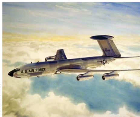
These two images show early configurations for a 707-based AWACS aircraft. The illustration on the left shows Boeing’s initial configuration for the AWACS, which featured a tail-mounted rotodome mounted on a forward-swept vertical stabilizer. On the right, the 707 aircraft featured eight efficient turbofan engines. Reduction in required endurance time enabled the standard 707 Pratt & Whitney engines to be retained.
