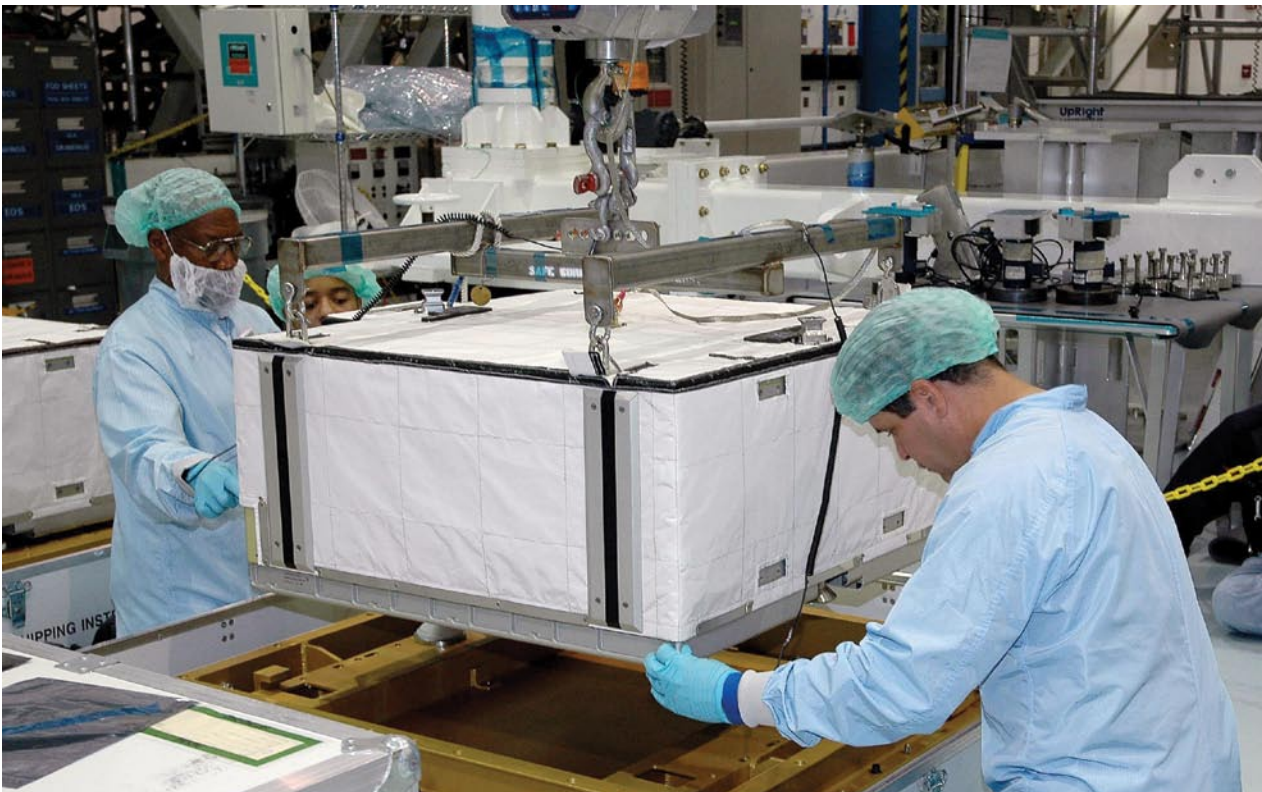
Elijah Walker (from left), Kyle Fears and Max Santiago, Boeing Checkout, Assembly & Payload Processing Services technicians, help guide one of six batteries for the P4 truss onto a stand in the Space Station Processing Facility at Kennedy Space Center, Fla. Fresh batteries were installed on the truss before launch.
