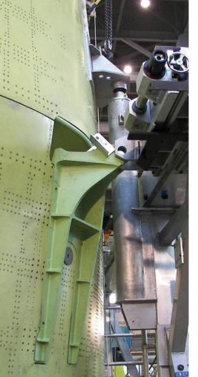
**Boeing Auburn Tooling Services produced** the main hinges (above) for the 747 Large Cargo Freighter's tail section. The facility thrives on complex work such as this, said Jeff Krueger, Auburn Tooling Services manager.
