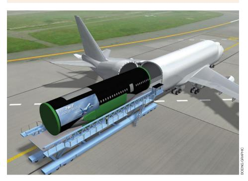
The 747 Large Cargo Freighter represents Boeing's commitment to new production-system methods on the 787 program. The LCF will transport large sections of the 787 airplane from partners around the world to 787 final assembly in Everett, Wash. It's the first time Boeing
