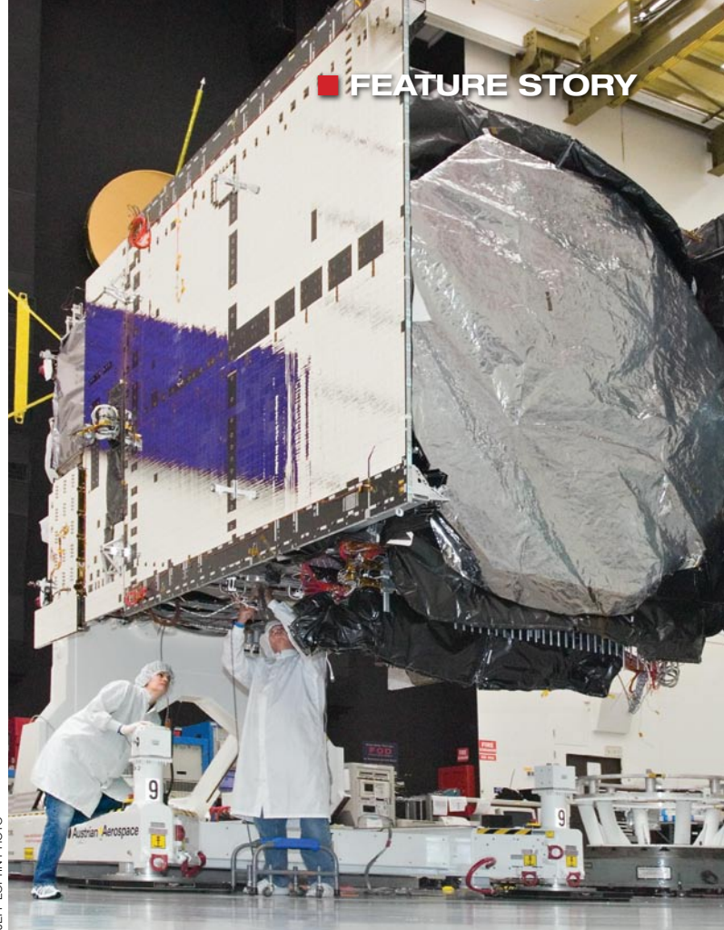
Boeing 702 satellites, like the one pictured here inside Boeing’s 60-foot High Bay in El Segundo, Calif., undergo final processing during this last stage of assembly and test. Once launched, these satellites will operate from geostationary orbit 22,300 miles above the equator.
