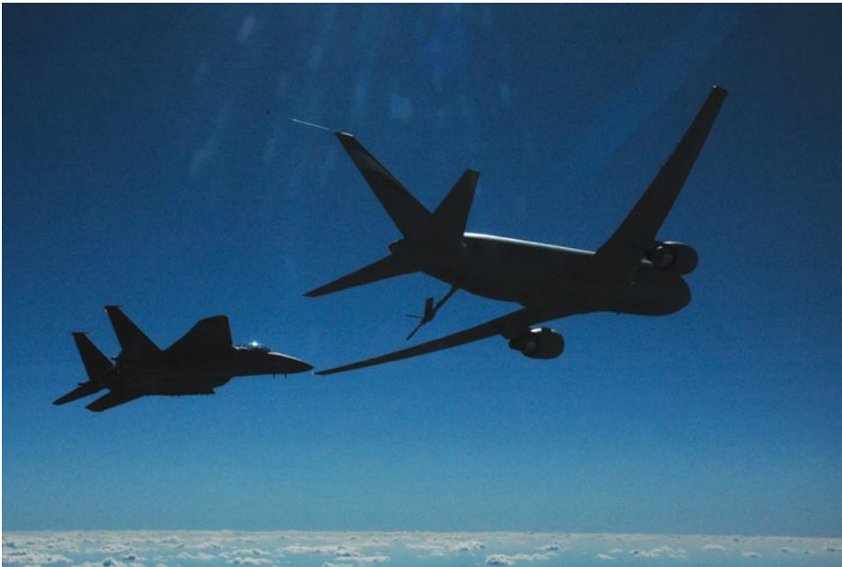
During a recent flight test, a Boeing KC-767 Tanker extends its fifth-generation, fly-by-wire boom telescoping tube as an F-15 follows in near-receiver position.
