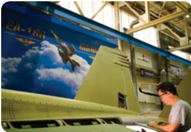
Brian Kuntz, a sheet metal assembler and riveter trims and fits a fairing on an F/A-18E/F in St. Louis.
