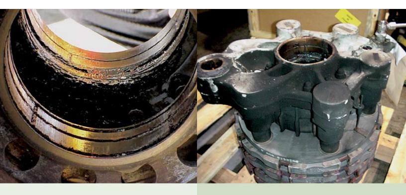
REMOVED BRAKE FOLLOWING FIRE FROM EXCESSIVE AMOUNT OF GREASE Figure 2
