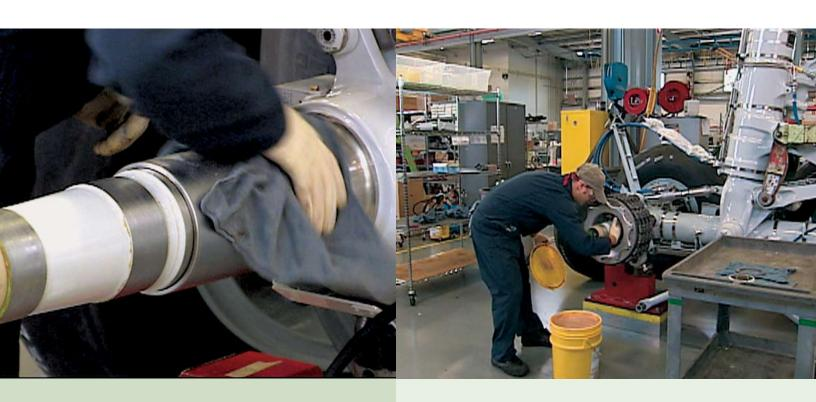
THIN LAYER OF GREASE BEING APPLIED TO BRAKE/AXLE SLEEVES Figure  $5\,$
